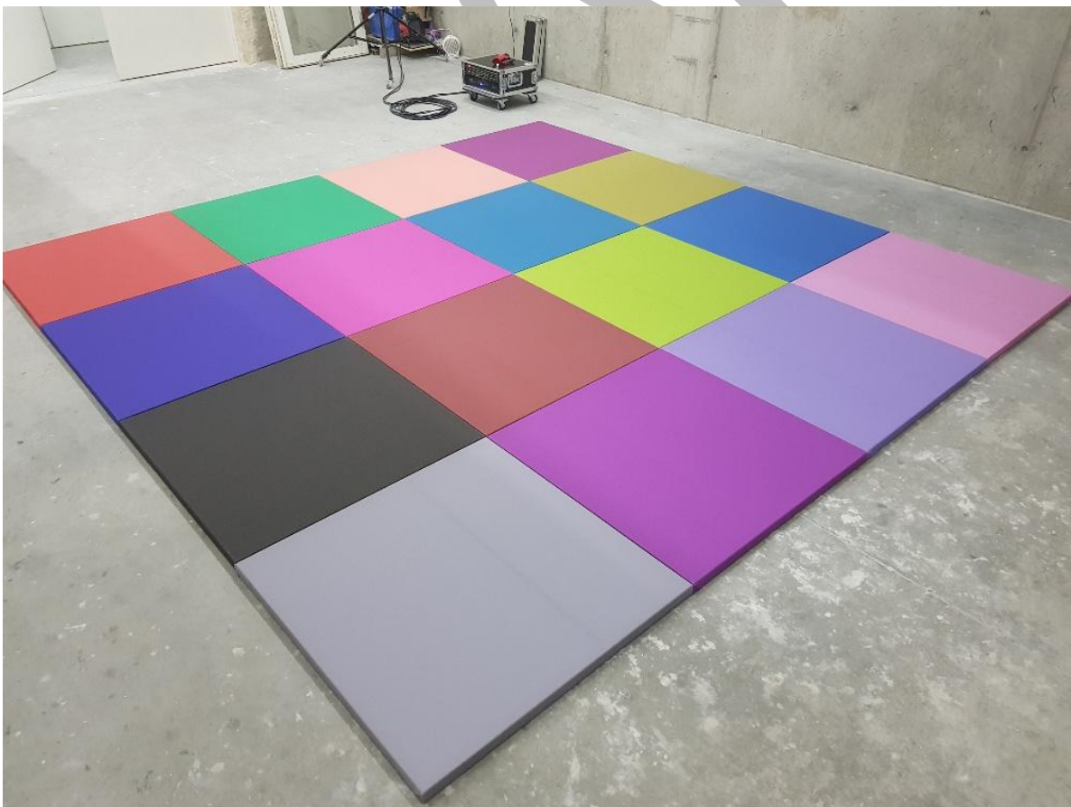
Figure. 2. Photos are presented the way of mounting of test specimen in the reverberation room. (16 panels were used)
